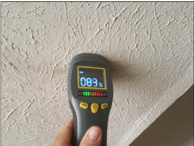
3.0 Item 2(Picture) Excessive Moisture
