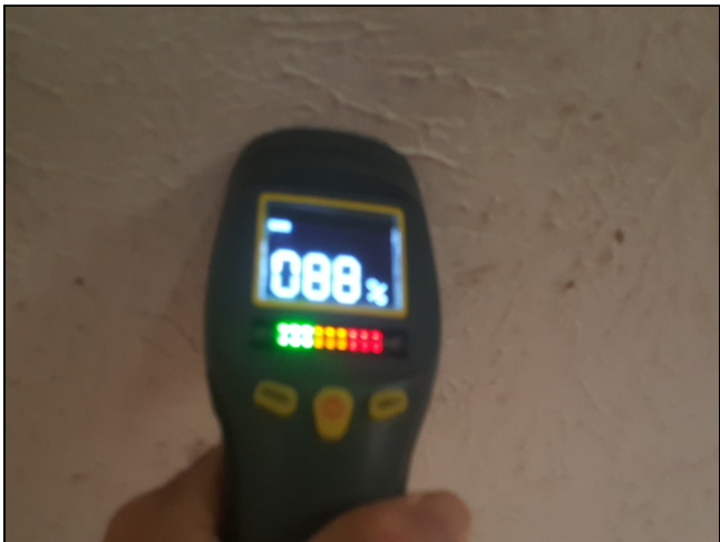
3.0 Item 1(Picture) Excessive Moisture
